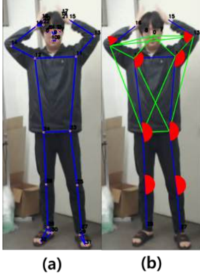
Fig. 1. Figure 1 (a) shows 33 joints information from BlazePose, (b) shows 35 pieces of joint complex information from proposed method.
